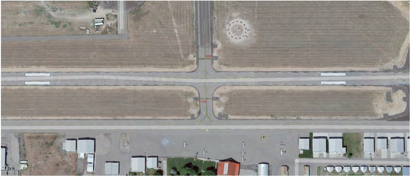
Figure 6.5: Runway 17/35, Taxiway C Intersection with Direct Apron Access
