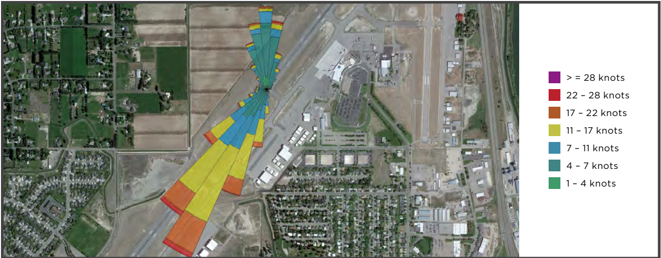
Figure 4.11: Visual Flight Rules Wind Overlay
