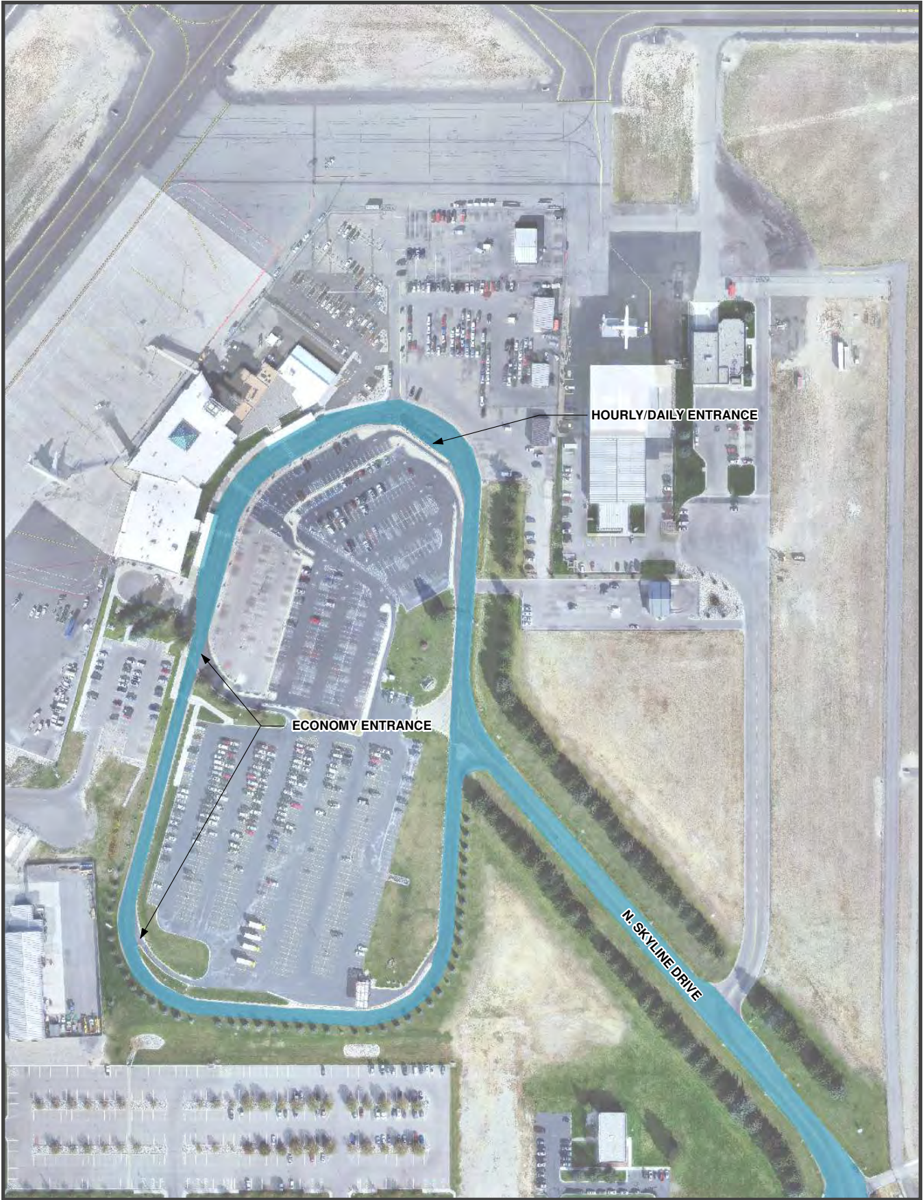
Figure 6.12: Terminal Roadway and Parking Circulation
